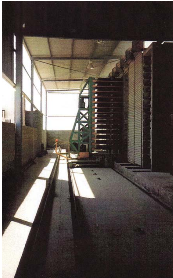
RAS Automated Transfer Car System / Finger Car with e.g. twin stack 2 x 14 nos
